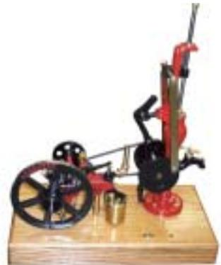
Pat O'Connor had a novelty engine. This tiny, single cylinder, compressed air engine uses an acrylic ball (from TAP plastic) for a piston.
