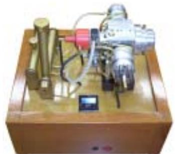
straight connecting rods pass through seals. There are only three moving parts making for easy maintenance and overhaul. See the web site; <http://bourke-engine.com> for a great deal of information about the early years of the Bourke and the more recent Melvin Vaux reincarnation of the Bourke.
