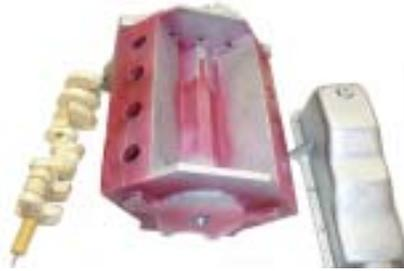
up crankshaft to go with the new five main-bearing V-8 project. He describes it as a "jig saw puzzle." The plan is to cast it in 4130 or 4140 steel with full counterbalances. Connecting rods, complete with balance tabs, are also planned.
