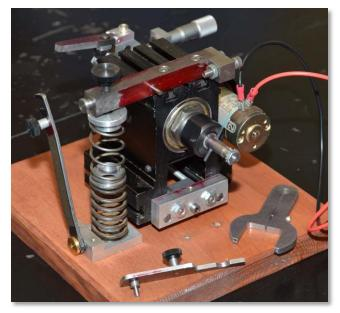
Carl Wilson demonstrated the Dover Cam Grinder. It is based on a Taig lathe headstock and will grind individual cam lobes for hit-n-miss engines or to be assembled onto a shaft for more complex valve gears. The Dover copies from a model lobe and is intended to be used with a wheel head supplied by the builder. It will be featured in a forthcoming article in Model Engine Builder.
