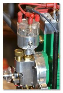
Outfitted with Dwight's new plug and distributor molded ends, the hightension leads look scale and have no leaks. The distributor cap is acrylic. The crankshaft is the familiar flat (180 degree) design, two up and two down. The motor is mount а welded up
