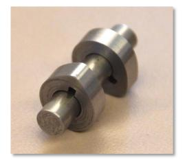
Cam lobes may be assembled onto a shaft to make a camshaft with multiple lobes. This method simplifies the construction of camshafts. In this example the exhaust lobe is in the foreground, the intake lobe in the background, and the camshaft rotates counter-clockwise.
