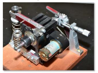
The drive motor is attached to the back side of the headstock and drives the spindle through a small vee belt. Grinding the cam lobe is controlled by the micrometer head which moves the model lobe follower in or out.
