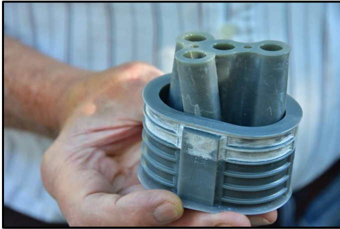
Jim Piazza-designed supercharger rotor and case, 3D printed by Mike Rehmus
