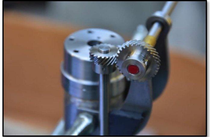
Peter's 48-DP helical-cut gears that were problematic
