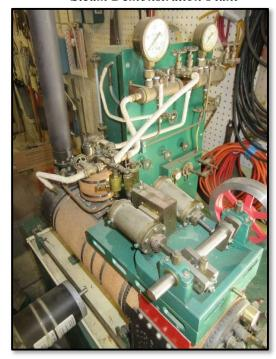
Henry Cranna, longtime member of West Valley Live Steamers, built this steam demonstration plant. It has a locomotive type boiler, twin cylinder oscillating engine, and a control panel. It was intended as an educational plant in how steam is generated, controlled, and utilized. Boiler operates on propane and a 5 gal tank is included. It is built on a shop cart with casters. Best offer.
