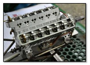
Mike Rehmus showed a number of 3-D printed parts associated with a small steam engine project he envisions powering with CO2 cartridges. He is using a Qidi i-box LCD resin printer. Mike reports parts have very good dimensional accuracy with the UV activated resin and modeling shrinkage in the solid model design.
