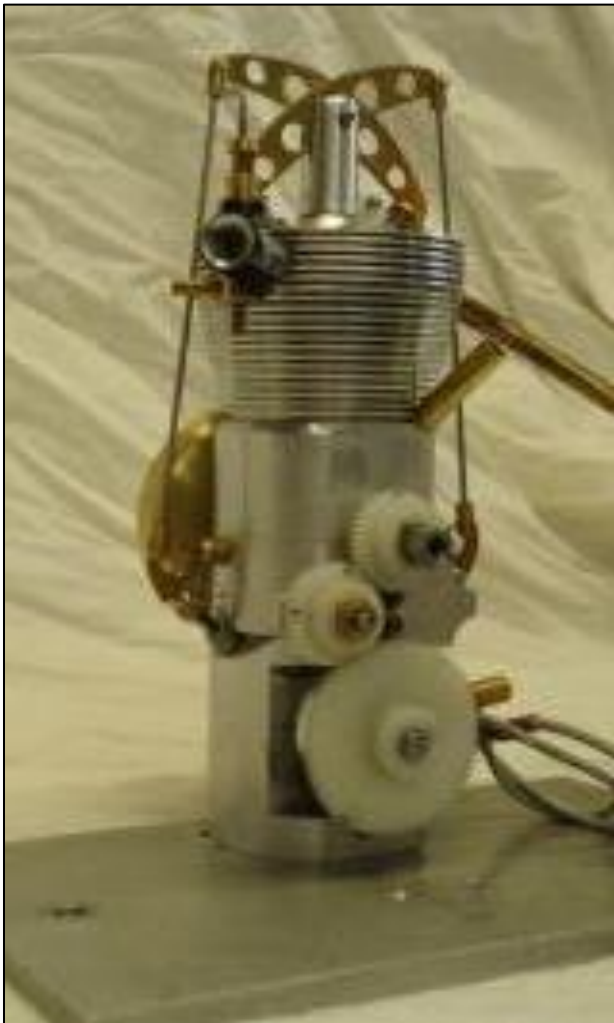
George Spain's original design single cam engine.
