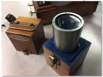
He next showed us a cylindrical square. The device is relatively rare and is called the Brown and Sharpe Precision Center. For highly precise metrology applications, this tool can very accurately measure a near-perfect ninety degrees.
