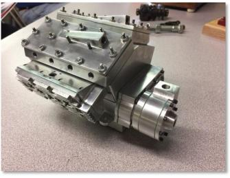
Joel Cohen brought us up to date on his "eight cylinder Seal Minor" project. He is building this from billet, as he prefers to avoid castings. Using the base dimensions of the original four cylinder Seal, he devised a forty-five degree V-8 with the help of his CAD program and a lot of imagination. The result will be a remarkable and unprecedented engine.
