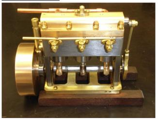
Jim Bove showed us a very lovely small engine that he based on an Edgar Westbury design of 1948. It is a steam engine that he runs on compressed air. It has a high-pressure cylinder that bleeds into a low-pressure cylinder. It uses model airplane engine cylinders and a rotary valve.
