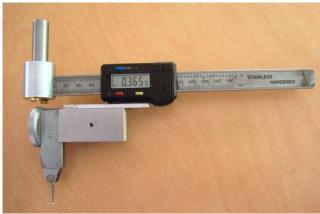
Jim also showed a nice center hole finder that couples a dial indicator mounted onto a six-inch digital slide caliper. The device mounts into a collet or chuck.
