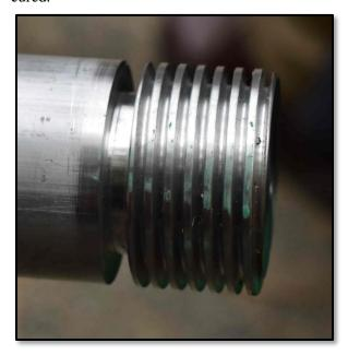
Dwight and Mike Rehmus are collaborating on an air cooled vertical GEM derivative. Mike brought in a piece of aluminum rod that had cylinder cooling slots cut. Mike attempted to cut the cooling fins as a continuous spiral instead of the conventional method of cutting individual fins. Apparently there were some issues involving broken cutters.
