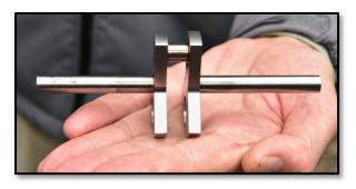
Peter Lawrence plans to show engines at the GGLS open house. He has a shop built Edison dynamo powered by a Stuart #9 steam engine which needed the new crankshaft. Peter showed the new crank with counterweights fabricated from O-1 steel rods and plate. He used V-blocks for alignment while the Locktite cured.
