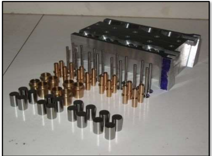
Duesenberg J-4 (four cylinder version of the original straight eight because "hey, I only have so much patience for 4-valves-per-cylinder engines!") with so many "itty-bitty" parts that the builder nearly had to check into rehab while making them (that's a Keith Appleton joke). Top side, in the foreground are the cam followers and bushings. The followers are hollow and fit over the ends of the valves. It's an overhead-cam engine: the recess milled into the front is for the timing sprockets and belts.
