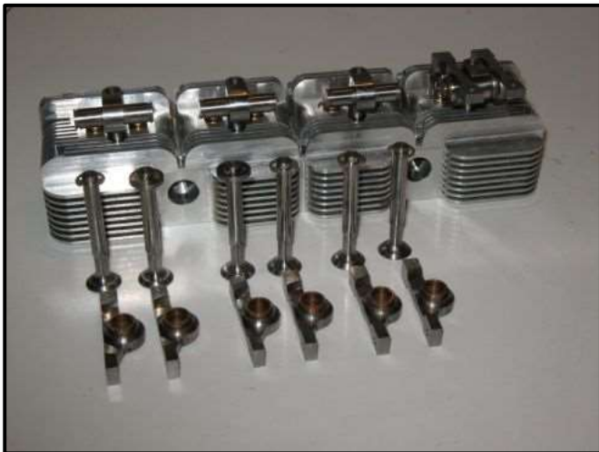
De Havilland Cirrus project - cooling fins cut and corner rounded, plus lots of "itty-bitty parts."
