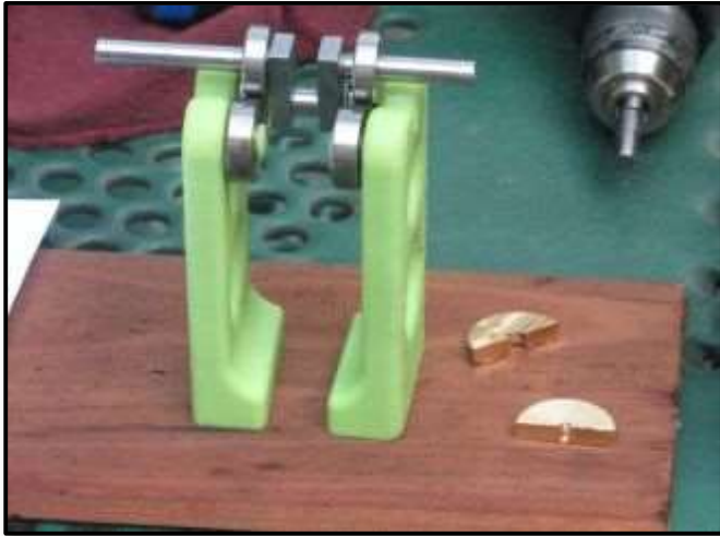
Mike's static balancing fixture with brass counterweights.
