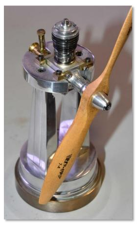
A discussion of the Schroeder Simple Single followed. This was an attempt to introduce a novice builder to a project that would likely result in a two-cycle running engine. It uses a Cox 0.49" cylinder, piston, rod, and head assembly. These are easily found and quite cheap. The Schroeder plans allow you to build a crankshaft, tapered collet for the propeller, crankcase, and back plate intake system. This results in a reliable runner.
