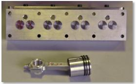
Dwight Giles has finished the rods and pistons on his very pretty in-line four project. He had to carve material out of the pan to gain relief for the connecting rods. The project is based on highly modified Wall Four castings. The 30 cc. design is now around 46 cc.
