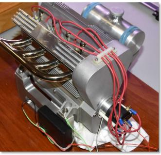
Paul Denham told us of his work with reed relays after blowing a number of Hall sensors on the Paul Bennett twin overhead cam four-cylinder engine. He then treated us to a run of the engine. It now runs great with a hot spark and has also been fitted with a new throttle arm allowing for a reliable idle. Paul says the reed relay functions exactly like a set of points and are durable and reliable.
