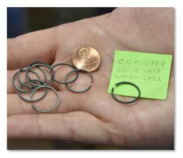
For heat-treating, Dwight has settled on 1200 degrees for an hour. When removed from the bag, the rings will show a dull red. The rings are then immediately dunked in cold water to achieve the desired temper.
