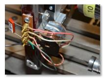
above) Two telephone ringer solenoids *See photo to the left. Think Ma Bell black rotary dial telephones – Ed.>* are the pickups for .detecting
