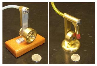
Mike Rehmus displayed two versions of the "wobbler" oscillating steam (or compressed air) engine initially developed for the WEME show. Dwight Giles made the prototypes. This engine will be featured in issue 23 of Model Engine Builder.
