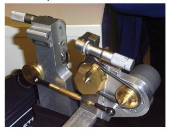
The work drive mechanism is mounted at the right hand side of the grinder. Starting at the right: the workhead drive motor and sheave; then a belt drive to the workhead spindle. The right hand center and dog drive pin are mounted on the workhead spindle. The masters are mounted at the right hand end of this spindle and are not visible.
