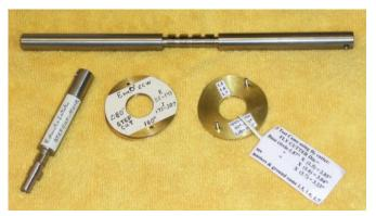
Bob displayed some of his camshafts and two of the masters. The masters (intake and exhaust) are soldered together at the lobe centerline angle and the pair of pins also operates as part of the indexing mechanism to phase the lobes for each cylinder. This is a simple and compact arrangement and works well.
