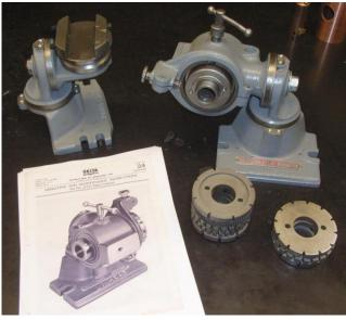
Anthony Rhodes is a knowledgeable tool collector. He showed the group a fine Delta Unihead UniVise (left) and UniHead (right). These work holding devices are commonly used for grinding tools at the various angles required for cutting metal. The vise is for lathe tools and the head for milling cutters. The division plates for the head are also shown. Anthony promptly received requests for a sale which he politely declined.
