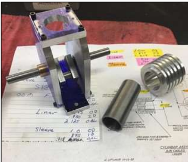
Snip of Upshur plate base assembly in process for an air-cooled engine
