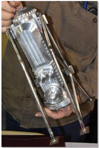
The crankcase has been machined and is now awaiting hand filing and smoothing. Peter does not use CNC for his projects, but says he couldn't be without a good digital read out. In addition, he has become a rotary table virtuoso, using various radius settings and fixtures to achieve a near CNC result. This engine has two oil pumps. One of the pumps seats into the bottom of the crankcase. Peter needed a flat base and ground a D-Bit for the application. End mills have a crown and are not suitable.
