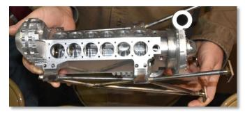
Peter Lawrence showed us a new tubular mount for his Rolls-Royce project. He used a TIG welder to tack weld the joints, then he silver soldered the remainder of the joint. However, he encountered problems with contaminated tungsten tips and the subsequent inability for the silver solder to flow. This will require tedious cleaning with a Dremel and a tiny bit. The "feet" of the mount were at four very odd angles. How to level them? He simply faced them off on abrasives fixed to a flat surface.
