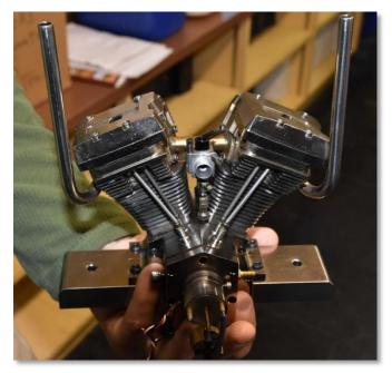
A builder in Oregon known to us only as "Virgil" made a very nice Harley style V-twin that needs a new connecting rod bearing. The construction was unorthodox and ingenious. The question was, "How do you tear this thing down?" After numerous members had inspected the engine and made suggestions, we had a clear idea of how to proceed. More information about this nice CNC engine is planned for subsequent meetings and newsletters.
