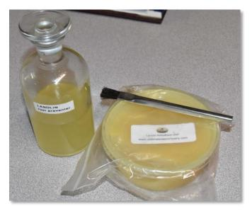
Do you need a potion to keep your tooling from rusting? Tim Horn shared an old timer's remedy for an anti-rusting application. It uses anhydrous lanolin as its base. This is mixed with 20% mineral spirits and is then brushed on any metal you wish to protect. Tim calls this "Nature's cosmolene from sheep". He got his supply from eBay for about ten dollars for half a pound or so. That should last for a few lifetimes.
