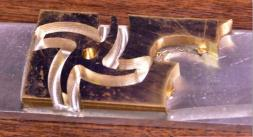
The brass water pump impeller was built by Mike Rehmus on his CNC mill. He had difficulty holding the work piece for an attack by a 9/64" sharp, 2-flute, new end mill. He finally
