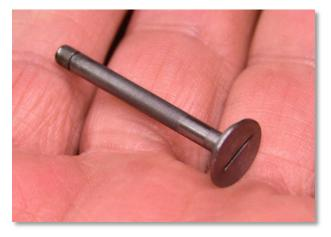
A smooth radius is placed between the valve head and stem to relieve stress. Also added is a small groove in the middle of the head is used to allow for a lapping tool access.
