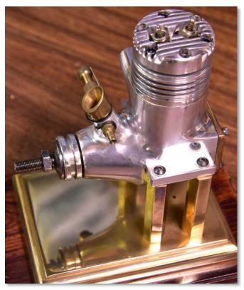
Bob Kradjian showed us his first effort at making a two-cycle engine. He employed a technique of taking a running engine, in this instance, a Merco .61, and replacing each part one at a time. After each part was fashioned, the engine was reassembled and run to confirm function.
