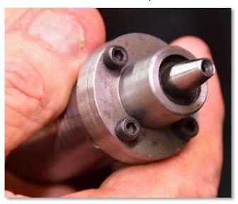
He uses a taper and a live center. He finishes and polishes the end opposite the valve-head first. The tapered cut relieves stress
