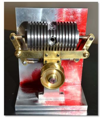
George Gravatt showed us his progress on his original opposed piston engine. He has now fitted a nifty curved-spoked flywheel and is arranging shafts, gears, cams, and a carb with a rotary barrel. Remember that all this building and designing stemmed from O'Connor's mock up of a Rootes-Lister engine. And, no; the red is layout dye and not the final color.
