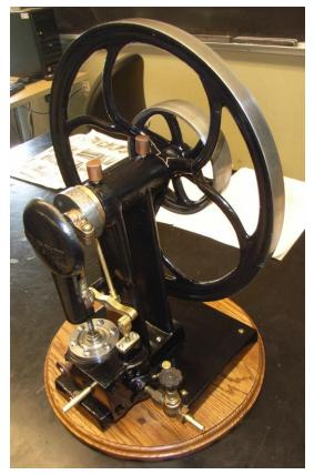
Jim Bove showed us a very pretty "Globe" steam engine. He found this in a very advanced state of rust, corrosion and decay. After extensive rebuilding, it looks lovely and runs on a low-pressure air supply. He re-did the cylinder, and repaired the connecting rod. It may have been a small, but "full-sized" steam engine for light duty application such as a sewing machine. Can someone give us a run-down on the Globe Company? It appears to be unrelated to the well-
