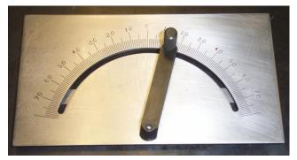
Dwight Giles made an excellent protractor to fit in the tool slot guide on a Baldor-type doublewheeled grinder. This steel plate device goes far beyond the simple miter gauges often provided with these grinders. It has machined surfaces, precise angle markings, and a clamp down to guide reproducible polishing and grinds.
