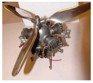
Jaime bought this Morton M5 in England. He has installed new rocker arms made from 4130 steel to the design of Bruce Satra and made a new engine stand.
