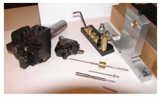
Steve Jasik displayed some special tooling for the lathe. On the left are commercially available box turning tools, commonly used on turret lathes. The workpiece is supported by the
