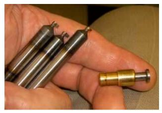
One of his special cutters was used to turn oring grooves in the tappet guides for a Wall 4 engine. The guide is brass and the tappet is the steel piece sticking out to the right. There was barely enough room to insert the boring bar into the guide to bore the groove.
