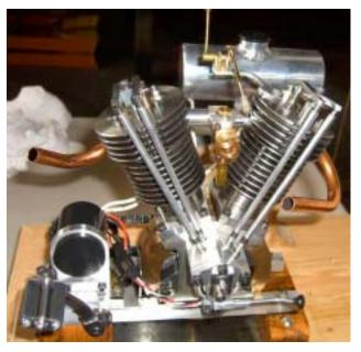
Bob Kradjian brought his Hoglet, designed and built by Randall Cox and modeled after a Harley-Davidson V-twin. It features Randall's typical open crankcase (the brass crankshaft cheeks are clearly visible.) Note the kick-starter made with a bicycle foot pedal. This engine uses two viton o-rings on the pistons: Bob noted that a new set of rings were recently installed. The neat aluminum gas tank is by our very own Paul Bennet.
