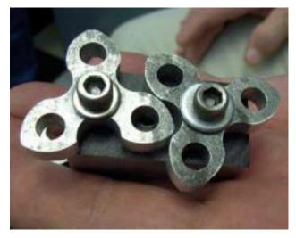
Pat O'Connor passed around his mock-up of a 3-lobe supercharger and pointed out the set-up and machining challenges and opportunities. Cutting the lobes was trickier than expected. He
