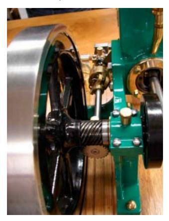
This view from the crankshaft end of this Vaughan engine shows the helical gears driving the side shaft and at the top of the shaft, the governor.
