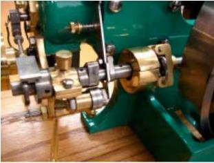
Another detail view, this time from the head end. At the right is the governor, middle the exhaust cam, and left, the igniter trip lever.
