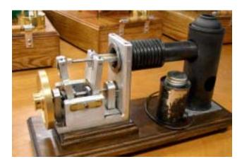
Al Vassallo displayed his unique hot air engine. Note the coaxial operation of the power and displacer piston, and the use of "found" materials.
