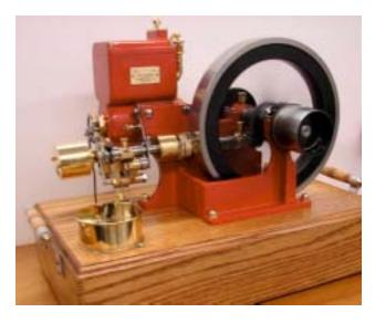
George Gravatt has his Vaughan engine running at last. He likes to make slight modifications to his engines to make them run better. His Vaughan was treated to heavier balance weights on the crankshaft and also heavier weights on the governor flyweights. The carburetor needle valve was threaded 5-54 to make fine adjustment easier. All three Vaughan engines are now finished and running.
