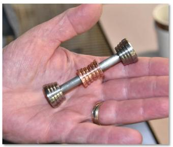
Lon Keeth showed us a novelty item that involved copper and magnets. It is a rod that has a ring that, when elevated, will slowly descend against all apparent logic. The magic is in the arrangement of the magnets and the use of copper.
