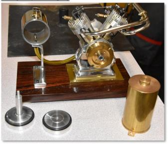
The secretary presented a quick and easy method for building a fuel (or water) tank using a threaded rod and two end plates with "O" rings. The photos are explanatory. Any tubing can be used with the usual arrangement for filling and outlet being threaded or silver-soldered. These photos can be seen in the March 2017 Crank Calls at the baemclub.com site.
