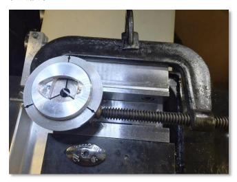
Steve describes the machining procedure, "The part is held in a 3" Hardinge step chuck which is held in a square 5C collet block in a (Kurt) vise. I needed a combination of 2 C clamps to keep the collet block from moving in the vise." The photo above is as Steve says, "Sometimes a vice is not enough."
