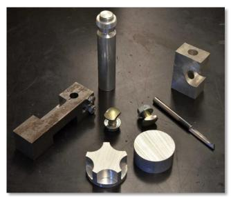
Jerry Franklin is continuing to make bits and pieces as he learns machine shop techniques. At a previous meeting he showed his external single point threading of a non-standard 13/16"-11 thread. Jerry made an internal threading tool from harden drill rod (on the right hand side of photo above) and threaded a matching nut. He made a replacement knob for band saw, hold down bolts for his mill from carriage bolts.
