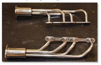
Dwight Giles showed a beautiful set of headers for the Black Widow made for Jim Kipp in Southern California. The aircraft stainless steel tubing with 0.028" walls is from "Aircraft Spruce". The flanges are 303 stainless made on a CNC machine in Southern California and pre-polished before assembly. A problem cropped up when it was necessary to "stagger" the pipes 5/16" to
