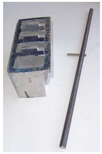
Don Jones is setting up to line bore the mains in the block of his Wall 4. He made a plate to fixture the block on the cross-slide of his lathe and the boring bar will be between the lathe centers. The tool bit in the bar is for illustration only. A shorter tool bit will be adjusted for size by a micrometer head mounted on a vee block.
