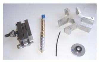
Steve Jasik is knee deep in building his rapid prototype machine. The brass and aluminum parts in the middle are blanks for the feed roller which grips and feeds the ABS rod to the right. The Aloris toolholder holds the feed roller while hobbing the teeth with a 3mm tap. The part at the lower right is the feed idler wheel. At the top right is a spider for holding thin work in a three jaw chuck. Magnets in the arm hold the spacer to the chuck and work is pressed against the spacer.
