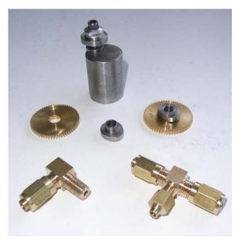
Dwight Giles brought a variety of miscellaneous pieces for display. At top center is a mandrel for eccentric turning of the flank arcs of an IC engine cam and immediately below it a cam lobe ready to be assembled onto its gear (60T at 48 DP) and finished cam and gear is on the right. These parts are for an Upshur farm engine. The brass flare fittings are copied from aircraft style fittings and are for his 4 cylinder Black Widow engine.
