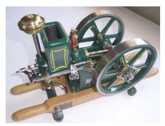
Bob Hettinger built this fine one third scale model of an Associated farm engine. It features a transistorized ignition system and spark plug rather than a magneto or low tension coil feeding an igniter.
