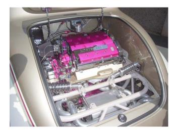
The extensive plumbing and wiring is not fully visible in these photos – you just had to be there to fully appreciate the complex layout and fantastic craftsmanship. John said that he mocked up the plumbing with wood dowels and hot melt glue before bending the stainless tubing.
