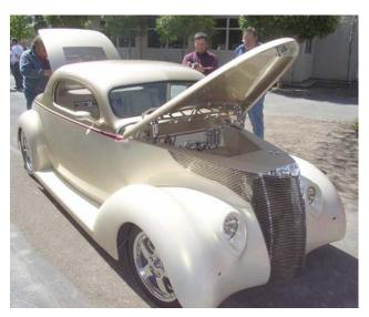
The Northstar engine was transplanted from a Cadillac El Dorado. Everything from the transaxle case to the wheels is John's design and fabrication. The two rear shocks are mounted in a unique position and are connected to the suspension by bell cranks and levers. The mufflers are located beneath the shock cross member and there is plenty of spaghetti leading to and from them.
