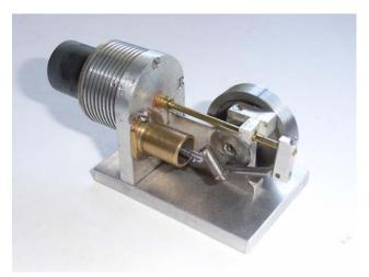
Mike Stimmann built this Stirling engine for his father, but it did not run when completed. Mike has since fixed it up with a stainless power piston and a displacer piston made from pumice stick glued to the displacer rod. Pumice is a form of volcanic ash and should be able to easily handle the temperature variations. It ran nicely on a small butane torch.
