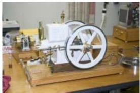
This bit of bright brass is Dwight's fuel tank made from 3" tube complete with a foot (check) valve to prevent fuel from flowing back into the tank.
