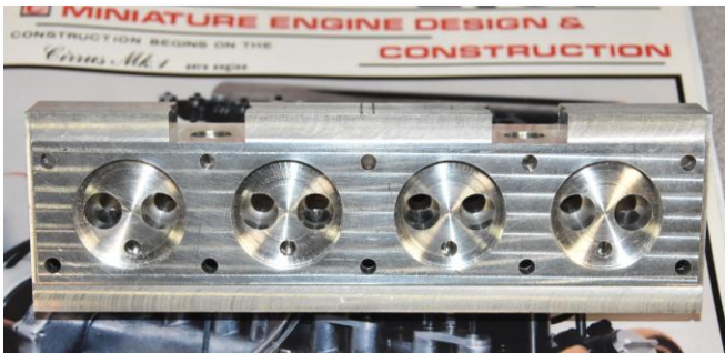
Peter Lawrence started a de Havilland Cirrus aircraft engine using Strictly IC plans. Project will be made from bar stock and Peter showed the machined head.
