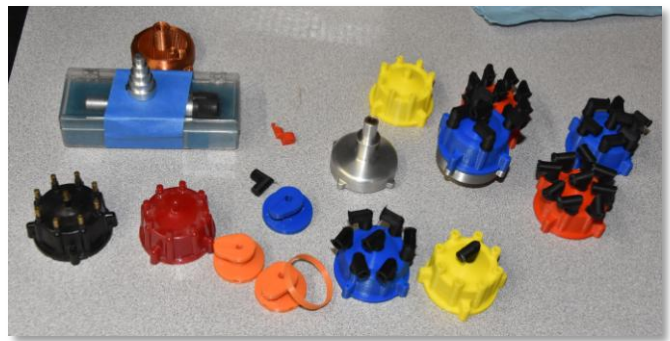
Mike Rehmus continues to explore additive manufacturing applications. He brought several examples of modular distributors that could be configured for 4, 6, or 8-cylinder engines. He also printed spark plug boots using flexible material.
