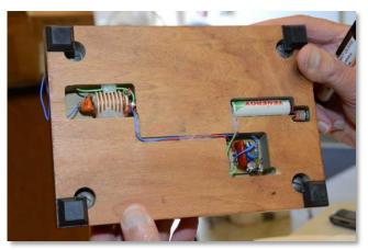
He also showed us the nine-dollar ignition coil that he removes from a commercial stove lighter. This would be for hit and miss engines, not multiple cylinder ones. If the engine is stopped with current on, there is no prolonged draw or heating of the coil.
