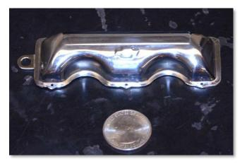
A sample of Jim Moyer's valve cover for his 1/6<sup>th</sup> scale 409 Chevy engine was passed around along with a display of its image on overhead projection. Jim told Paul Denham that one of the hardest parts of making his historic Corvette was the oil pan with the deep draw required.
