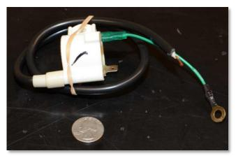
An ignition coil found on e-Bay should work well for us. It costs \$7.00 and is probably intended for a "weed-wacker" engine. While probably best used with CDI, it should work with coil and condenser.
