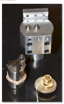
Dwight showed us the centers for a crankshaft fixture. It uses four separate pilot holes. He also told us about a method for cam lobes that can be cut on a lathe quickly and easily.
