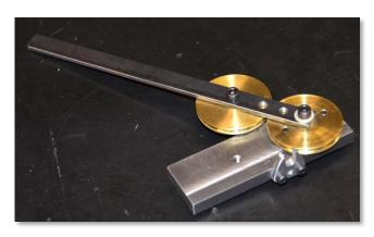
A commercial customer needed six protective bent rod cages for expensive sound sensors. Dwight adapted some scrap discs into a shop-built rod bender, and gave us a demonstration. It was quick and easy, resulting in perfect bends. For the headers on the Black Widow V-8's he used a bender with two separate radiuses (radii for you Latin scholars). Thin-walled stainless was the material used.
