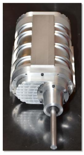
Jim Freel is now working on the supercharger for his V-8 build. The end caps and blower block are machined from 6061 aluminum on a three-axis CNC machine.
