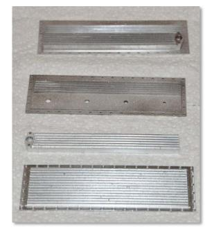
Jim Piazza showed us some very fine work on the side plates described for Ron Colonna's 270 quarter-scale Offenhauser engine. Using a build-up of two pieces and Lock-Tite for the plate, Jim used a 1/16th end mill and his 3-axis CNC mill to cut the flutes. This resulted in a finely detailed pair of side plates. For additional information, he was able to see and photograph a Root's-Blower supercharged
