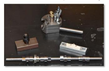
Four"). His efforts have been bolstered by the a Little Machine Shop CNC milling machine. He has been fashioning the rocker arms and cam lobes using Alibre and Mach III.
