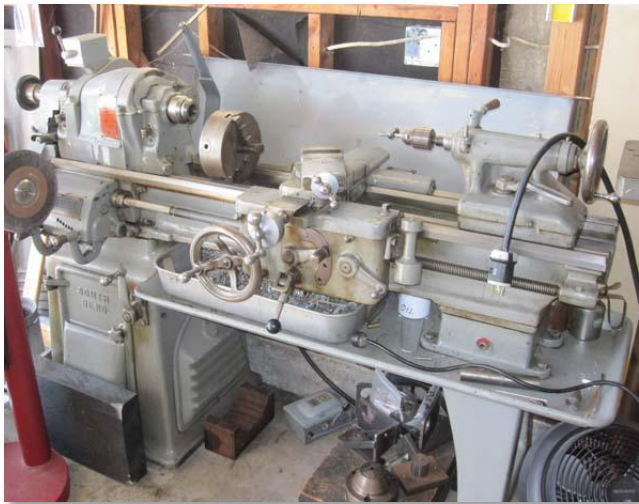
SOUTH BEND LATHE, BELT DRIVEN, MODEL C/L 145B
