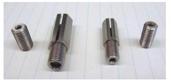
Steve Lawrence was having difficulties holding short turned studs in stainless steel. He decided to take hex stock, bore and thread it. Following that, he slit one of the faces. When the stud is threaded into the hex, clamped into a three-jaw chuck it chases the threads quite nicely and can be firmly grasped without marring the threads.
