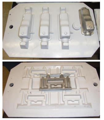
The match plates for the oil pan and the intake manifold were on display, as well as a finished casting of the pan. The quality of the pan casting is remarkably good. There is no visible porosity. Dwight and Ken located a foundry in San Jose who produced the casting. It is:
