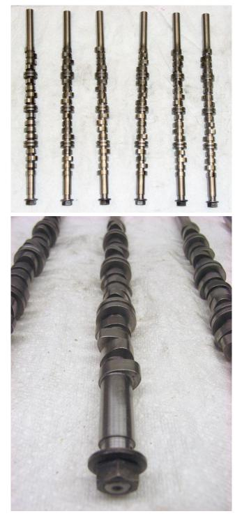
Camshafts: Dwight's home brew heat-treating method is worth noting. He chucks the shaft in a slowly turning drill press and heats the top four lobes with a torch to a cherry red. Then he dunks it, straight down, into water. This process is repeated on another batch of lobes, with minimal distortion resulting. Jim Kipp, in separate development in Southern California is working on a CNC'ed block for the Black Widow.
