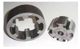
Peter Lawrence doesn't mind doing things the hard way! These are the stator (l) and rotor (r) for a dynamo – that is, a DC motor or generator. The stator is from a slice of thick walled tube and the rotor is from solid bar. The pole pieces in each have been formed by a combination of drilling, milling, and filing.
