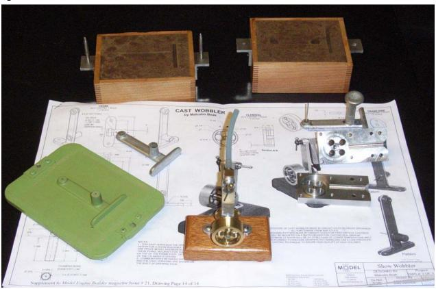
The photo above is an overview of the "Show Wobbler" engine commissioned by Mike Rehmus, and designed by Malcolm Beak. Plans and construction notes are in issue #21 of Model Engine Builder. Beginning at the lower left of the photo: the green rectangle is the pattern
