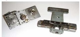
Anthony Rhodes displayed this very unusual saddle and apron from an Atlas/Craftsman 6" x 18" lathe. The original apron is part of the saddle casting: here it has been cut off, the saddle modified to fit the bed, and a complete new apron built complete with power crossfeed. This has to one of the very few of these lathes with this modification.
