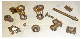
Roy Anderson made the patterns and the lost wax casting for simplex steam feed pumps in two sizes: 1.5" x 1.5" x 1" and 1" x 1" x 5/8". I'll go out on the proverbial limb and say that those dimensions are steam cylinder bore x pump cylinder bore x stroke.
