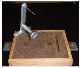
The casting above is "right out of the mold". It is resting upon the cope (upper) half of a mold made from Petrobond sand rammed up on the pattern board. The molten metal enters the mold through the pouring basin (conical shape that extends the main bearing boss) and runs through the mold. The displaced air exits the mold through a vent hole. The thin rod at the top of the casting shows that the metal was sufficiently fluid to fill the vent hole almost to the top of the mold.
