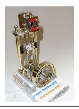
Rick Levesque has completed another in his series of superb steam engines – the "Little Workhorse Engine by Rudy Kouhoupt and featured in the July 2000 Live Steam magazine. Note the unusual cross-head and guides. Rick said that alignment of the engine was a problem: "it is one thing to make parts, making them run together as an engine is something else." Congratulations Rick on a fabulous job.
