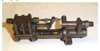
A shuttle valve (top left) operates a steam valve (middle left) via the lever in the middle. The steam cylinder (bottom left) drives the single acting pump cylinder (right.)
