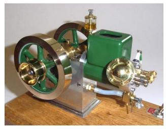
This is Dwight Giles' build of the Upshur farm Engine from plans in Strictly IC magazine. Dwight said that other than some details, it is as originally designed. But the devil is in the details: throttling carburetor, 5 bolt head, counterweighted crankshaft, muffler, gas tank in crankcase, caps on main bearings, and cast flywheels. Looks like it is about ready for First Pop Honors next month.
