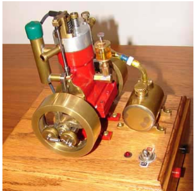
George Gravatt's Little Devil with water-cooled cylinder.
