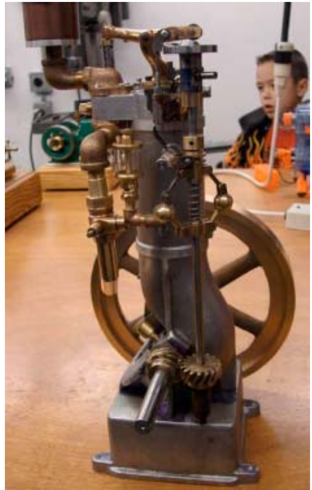
Dick Remington is also making a Red Devil and it looks almost ready for its first pop! Some of the unique features of this engine are clearly visible. Starting at the crankshaft: helical gears driving the tower shaft, partway up the flyball governor, and at the top a face cam operating a cam follower. The flywheel on this end of the crankshaft has been removed to make these details easier to see. Also note that the intake and exhaust valves are located in a chest to the side of the cylinder. For more info on this engine: http://www.shelfpetmodels.com/
