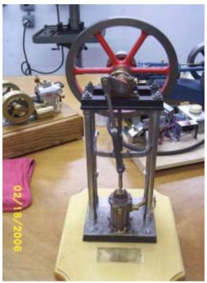
Robert Schenk showed his build of the PM Research double-acting steam engine. This was advertised in the 1895 Strelinger catalog as a 1/4 hp portable power engine. It features a 1.5" bore x 2.5" stroke in a double-acting cylinder, and a piston valve.
