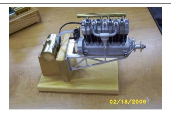
Here is John Meredith's Sirius, a Merritt Zimmerman designed 1/5<sup>th</sup> scale model of the De-Havilland Gypsy Moth 4 cylinder in-line aero engine. John has installed glow plugs in the head and will later change them for spark plugs. He said that it took quite an effort to find the proper angle to drill the plug ports, not a lot of room. Another challenge was the very small camshaft that was ground from the solid.
