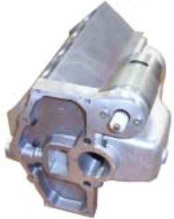
I brought Alan Ingersoll's historic Curtiss Model D12D. This V-12 is a 1/5 scale model that Al carved out of billet. He cut no corners with this project which has overhead cams driven by bevel gears, a propeller drive gear ratio of
