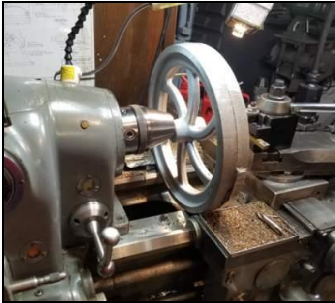
Flywheel casting barely fits on Paul's lathe
