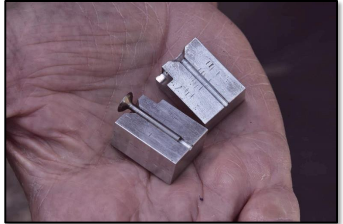
One of the 48 valves in the valve-head slotting jig
