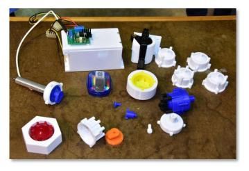
Mike Rehmus is continuing to evolve his additive manufacturing product line of model engine distributors. He has versions suitable for 2, 4, 6, and 8 cylinder engines. This month he had an operating prototype showing rotor function and a printed fixture for machining commercially procured distributors.
