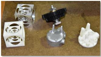
Mike Byrne discussed learning to produce scalable parametric models in Solidworks. Examples were a Turner's Cube with recursively smaller bores and a spur gear program that will produce correct involute geometry for specified number of teeth, diametrical pitch, pressure angle, and whole depth ratio. He showed 3-D printed "proof of concept" examples.
