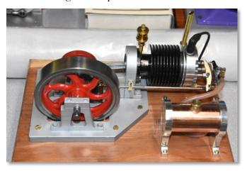
A second showing was his Jerry Howell engine. He fitted it initially with a TIM 6 ignition system. It sputtered a few times and then totally failed. A CDC device was substituted, now it promptly started and ran well. He then made a nice demonstration of the engine's running.
