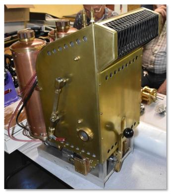
Charlie Reiter made a steam engine for a bicycle! The boiler and engine are in one 70-pound unit. A Coleman burner supplies the heat. He modified a
