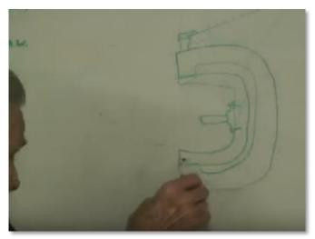
The attachment frame is made of steel. The cutting tool depth is set with a separate micrometer attachment made of aluminum which uses magnets to attach it to the steel ball turner frame.
