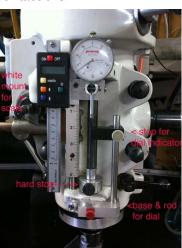
Steve Jasik described a fixture attaching for digital slide caliper for the quill of his vertical mill. It is nicely made of white plastic from batch that Roy Anderson had given away at a previous meeting.
