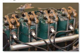
The Champion V-3 plugs are original. In 1985 the Cole's catalog listed the casting set for \$165 and the plans for \$13.00. This engine has a tendency to sling oil from the exhaust. Adding small scoops to the rod caps, and lowering the oil level can mostly cure the problem.
