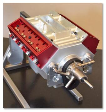
Jim Freel has completed the cylinder heads for his Black Widow V-8. The valve guide cages also serve as the seats. The intake manifold is a lovely piece of jewelry requiring about five hour of CNC machining. Jim uses a combination of conventional manual and numerical techniques to fashion his components. The crankshaft and camshaft construction is next for this beautiful build. The water pump is a Giles design. The anodizing on this engine was by Santa Clara plating.
