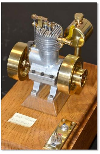
Dwight Giles built a Bob Shore's design back in 2005. He built a new gas tank and modified the flyweights. The only remaining work to be done is the Hall-Effect timer and electrics.
