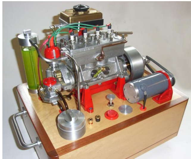
Dick Pretel has once again worked his magic on an engine built by someone else: this time a Wall 4 by Frank Kurtz, an Ampex machinist, now deceased, and a member of BAEM. Dick installed a C&H electronic ignition, a scavenge oil pump feeding into a tank, and a pressure oil pump feeding the bearings in the engine.
