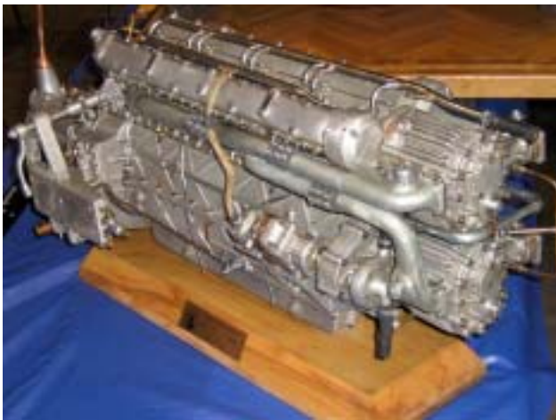
Flore Di Bernardo built the Maserati Tipo 8CL straight 8 seen at NAMES. Note the fine level of detail in the sand castings.
