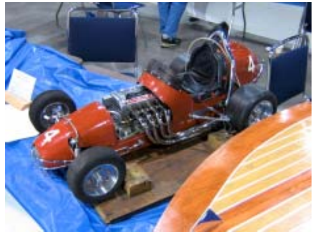
James Riggle put his Novi V8 into a midget car and the OHC 4 into a speedboat.
