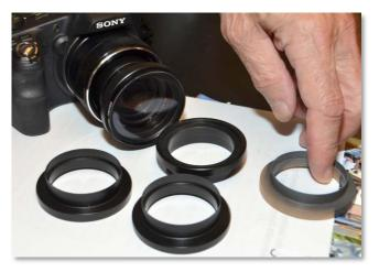
Steve Jasik bought a nifty new Nikon camera that did not have a filter ring adapter. That's not a problem if you have a CNC lathe. This is a 13 thousands affair with a half millimeter thread. Steve made a couple of these delicate and precise rings.
