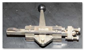
Roy Anderson showed us a nifty engraving tool. He used this to mark crisp division lines for hand wheel hubs. A spring gadget returns the cutter to the starting position. Short and longer stops limit the scored lines to major and minor divisions. It all makes for very nicely done tool.
