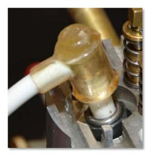
Here is the finished boot in its place atop the spark plug.
