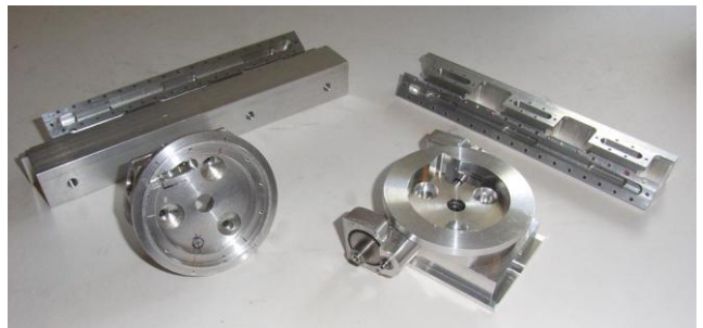
The top two pieces are partially completed intake manifolds. The slots in the right hand block are the visible part of the intake port which is a 90° elbow within the block. Peter machined these by milling successively deeper cuts at increasing angles from both sides of the port. This left a small web in the center which was removed with a rotary tool. Design changes to the intake manifolds and assembly problems required new supercharger parts (bottom of the photo.)
