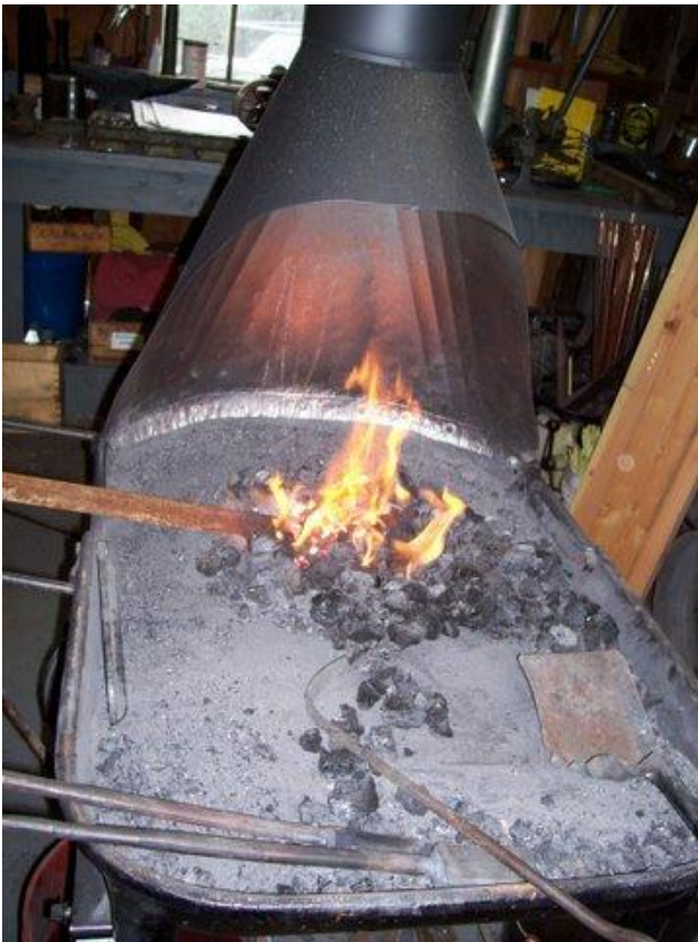
The top photo shows heating the workpiece in the coal fueled forge.
