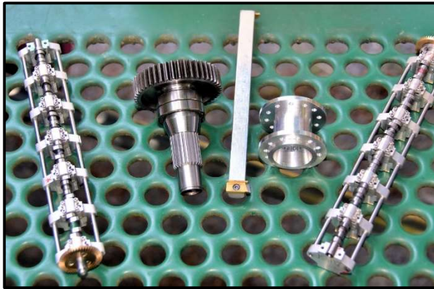
Peter's finished camshafts, prop shaft, prop hub and shop-made broaching tool.
