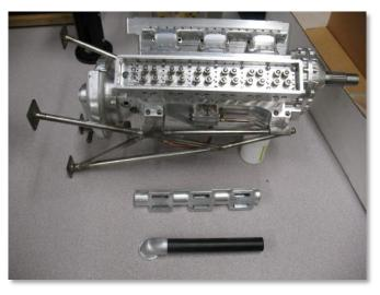
Peter Lawrence brought his Merlin. He described process for removing a broken 2-56 tap using hydrochloric acid (needed despite his regular use of Tap Magic). Other new Merlin parts were an induction tube, super charger carburetor, and an exhaust exit elbow. He also mentioned a Duisenberg candidate project. He has acquired some scanned drawings that are available on the BAEM web site ).
