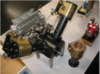
Charlie Reiter showed a 1920's brass wobbler 4 cylinder Gunderson boat engine. He also had part of a 2 cylinder Heisler locomotive engine.
