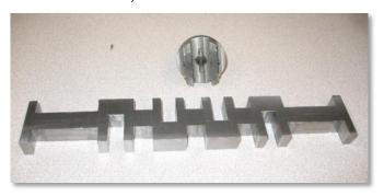
Dwight Giles brought in a 4140 4-cuylinder crank blank and a fixture for turning crankshafts. The fixture mounts in a collet and drives the work without a lathe dog. He also descried his turning workflow.
