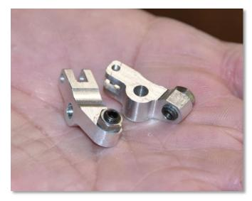
Paul Denham made a batch of 32 rocker arms out of aluminum tooling plate. They developed cracks around a narrow rim surrounding a 10-32 threaded hole. Next, he went on to another set of 32, this time from 6061. This also, was not strong enough and showed weakness. The final set was from 2024 and made the grade!
