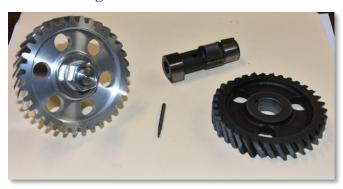
In a recent shop visit, Dwight Giles showed Paul an antique Johnson four-cycle engine. When attempting to turn it over they discovered a badly stripped-out gear. It happened to be a 12-diameter pitch, 34 tooth, left hand, and 30 degree helical gear. Now, since Dwight turned out aluminum blank and Paul had a four-axis milling machine, what would prevent him from machining a helical gear? The G-Code for this task was from Gearotic. Each tooth requires three passes, one creates the root, another
