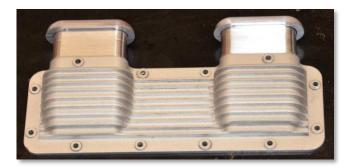
Jim Piazza is continuing with various parts for a small scale Offenhauser 270 engine. This is the side-plate breather. It is nicely done with a bead blasted finish. The fins required a good bit of
