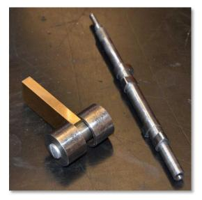
Joel's engine, which is made from the solid, looks a bit like Mason's "Mastiff" but has twin carburetors and twin camshafts and generally is better finished. The Mastiff uses a single camshaft. The connecting rods are not staggered and use a "blade" style arrangement at the big end (mockup on left in photo above). The ignition system is next on his building schedule.
